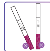
Fig.3 Never hold the test strip with the sample pad pointing upwards during testing
